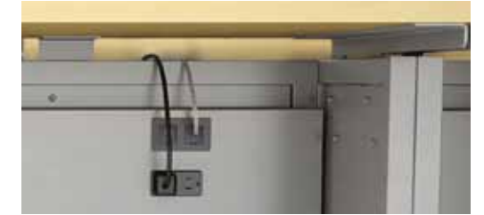
POWERLEX BELOW (Non-Sequential Daisy Chaining) Powerlex embedded in Impression offers 2 duplex receptacles, 4 data openings, a voice/data kit for customer-supplied jacks, 2 quick-connect jumper cables and enclosures. Building power is accessed via hardwire to the building followed by up to 12 units in any order.
