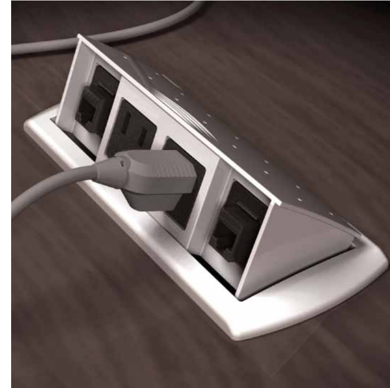
MINIPOINT BELOW A great power and data solution for everyday needs. A fluid pop-up feature presents connections for your daily meetings. The 3" x 7" product comes standard with 2 receptacles and 2 data openings. A six foot power cord, 15 amp capability, and a voice/data adapter kit for customer-supplied jacks are included.
