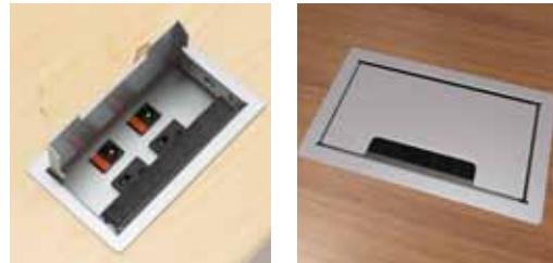
VILLA ABOVE AND RIGHT (Non-Sequential Daisy Chaining) Our #1 selling power and data solution, this unit comes in two versions: corded with convenience outlet on bottom or hardwired with 2-circuits. Each grommet is 3.3" x 5.5" and comes with 2 receptacles and two RJ-45 CAT6 punch-downs or just 2 receptacles.
