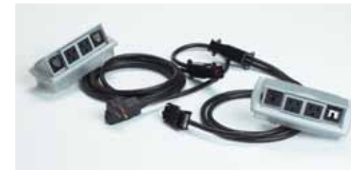
MINIPOINT ABOVE (Sequential Daisy Chaining) Less expensive than non-sequential daisy chaining, this product allows you to connect multiple tables. Up to 8 Miniports may be connected in a sequential fashion. The first unit has a 10' power cord and 6' interlink cable. Color coded interlink cables provide a "dummy proof" connection methodology that ensures a safe electrical connection for all succeeding tables. Units 2 through 8 must be connected in a specific order.
